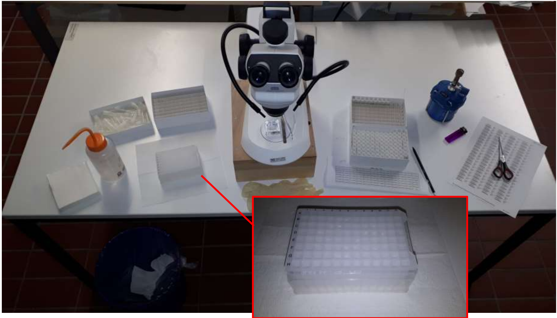
S-block filled with ATL buffer and Proteinase K and silicon pad
